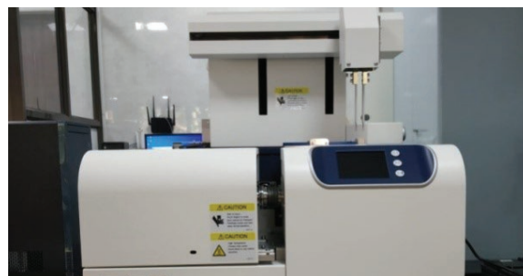
▲ Thermogravimetry/ Differential Thermal Analyzer (TG-DTA) Model: NEXTA STA300, Hitachi, Japan
