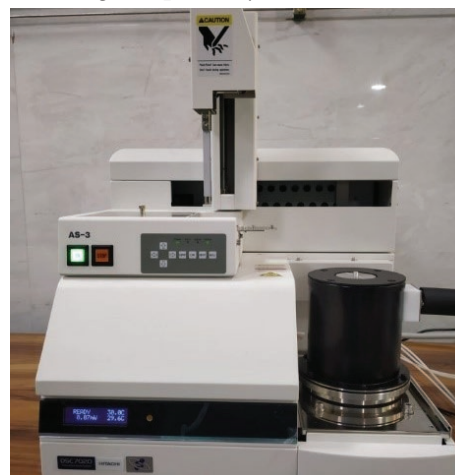
▲ Differential Scanning Calorimetry (DSC) Model: DSC7020, Hitachi, Japan
