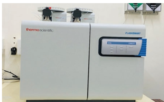
▲ CHNS (O) Analyzer at SAIF/ CRNTS Model Flash smart V CHNS/ O, Thermo Fisher Scientific Pvt. Ltd., USA
