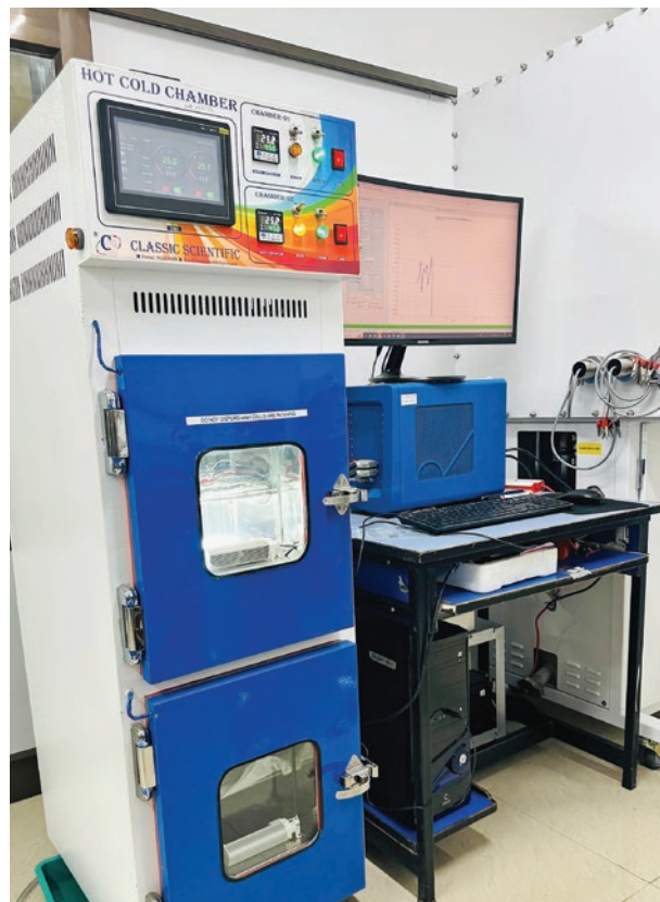
Temperature controlled battery characterization setup
