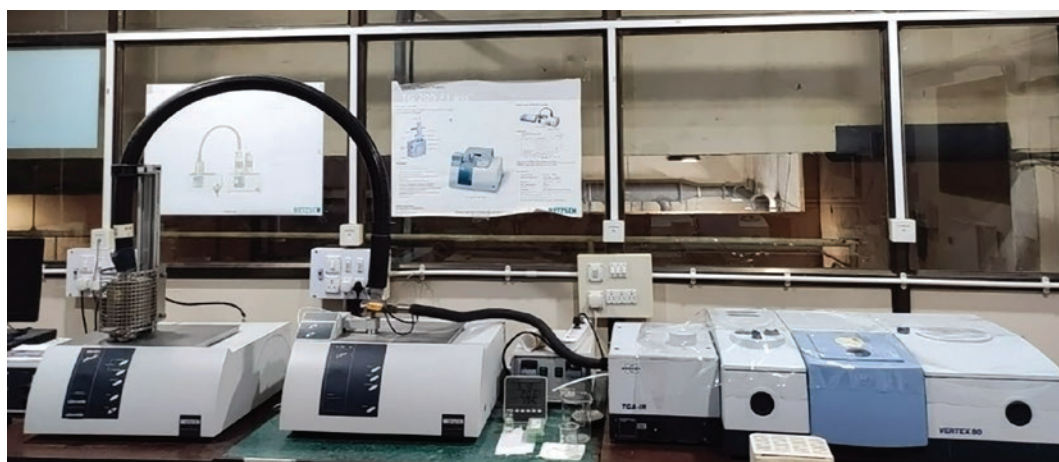
Thermogravimetric analysis (TGA), Fourier transfer infrared spectroscopy (FTIR), mass spectroscopy (MS) setup
